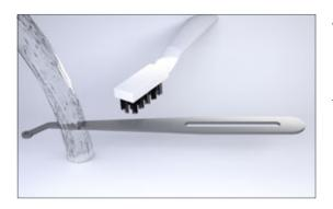
**Automated procedure:** All multi-piece instruments (i.e. Distance Indicators, Ratchet and Torque Control Device) must be disassembled into their single parts and pre-cleaned with a soft nylon brush under de-ionized water until no contamination is seen (use magnifying glasses 3x).
